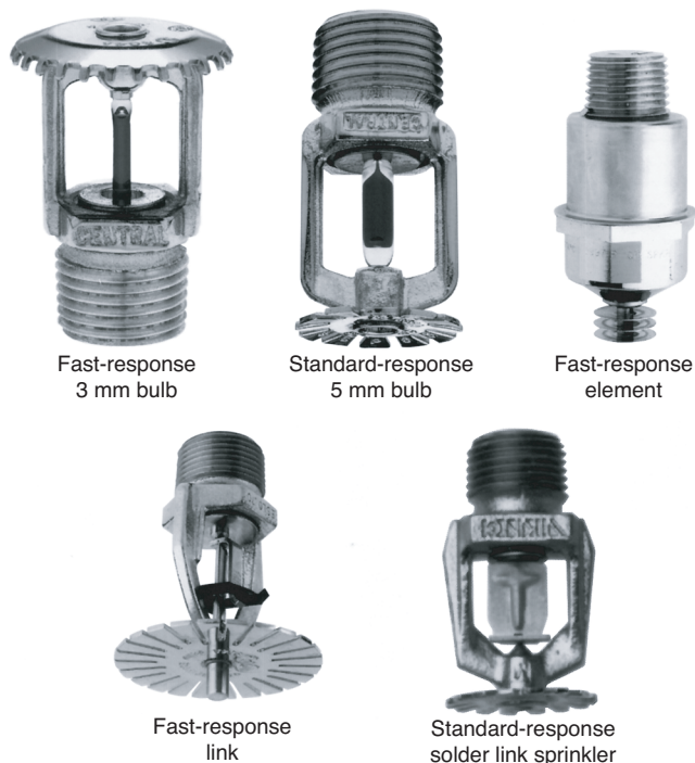
FIGURE A.5.3.1.1 Sprinkler Operating Element Identification.
